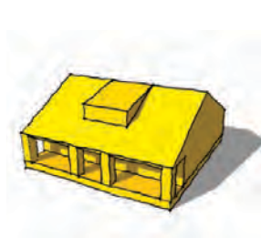
A 1 1/2-story side gable
